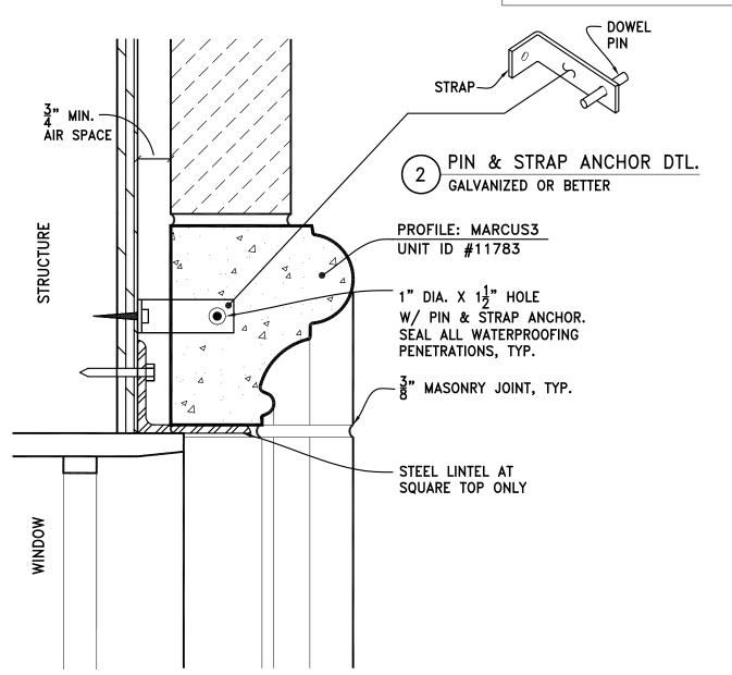
CAST STONE HEADER ATTACHMENT AT MASONRY VENEER WITH PIN & STRAP ANCHORS
